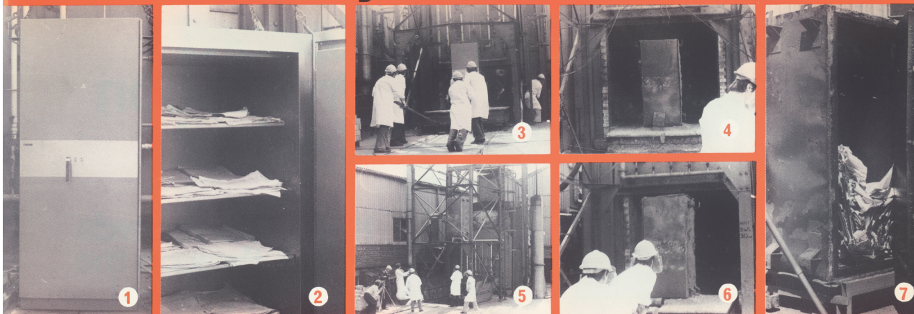
Explosion Hazard and Fire Impact Test: (1) Cabinet ready for insertion. (2) Shelves lightly loaded with paper. (3) Inserting into blazing furnace. (4) Removal from furnace. (5) Raising for drop test. (6) Returning to furnace. (7) Test papers, although creased from drop test, undamaged by heat.
